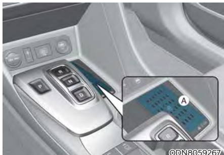
[A] : Wireless Charging Pad (In-vehicle Authentication Pad)
