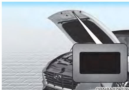
Air conditioning refrigerant label
