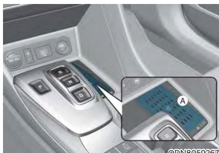
[A] : Wireless Charging Pad (In-vehicle Authentication Pad)
